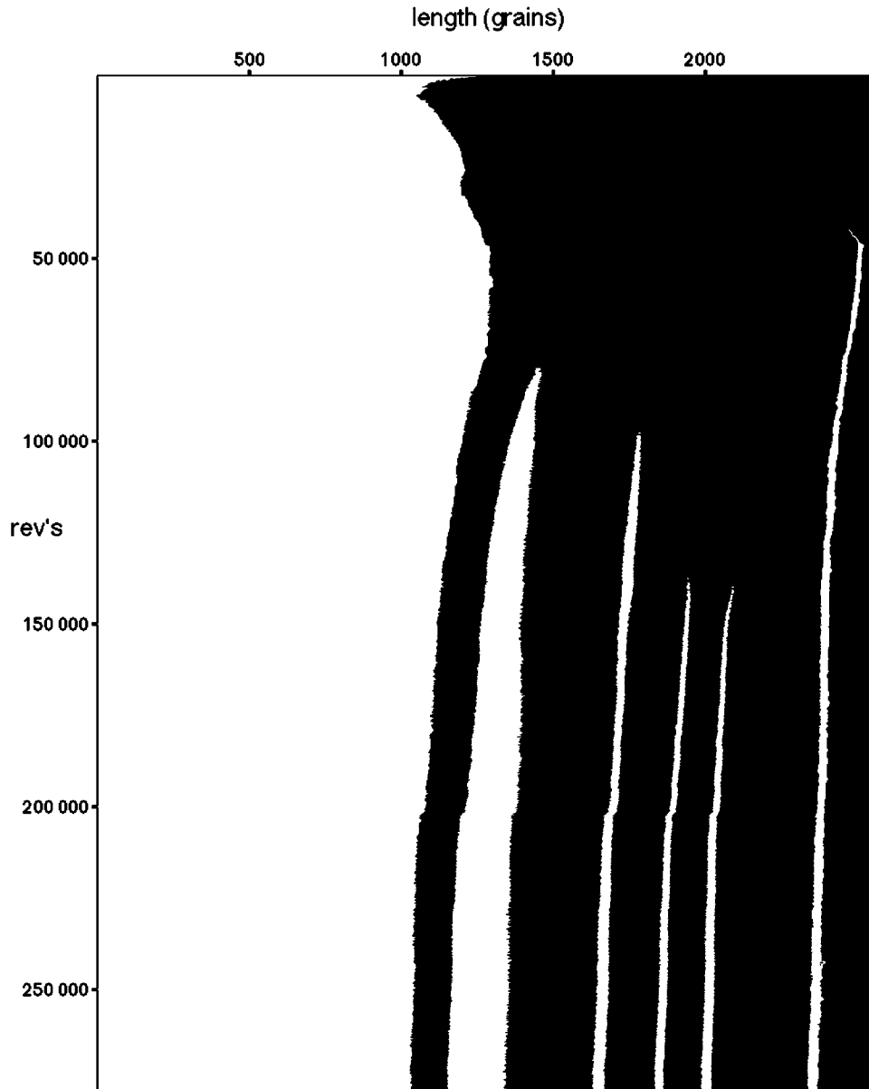
FIG. 5. Space-time diagram for the experiment specified in Fig. 3. The distance along the tube is given in terms of the average sand grain diameter. The diagram covers 326 h (278 000 revolutions).
