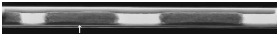
FIG. 1. Horizontal tube ( L = 16.2 cm) half filled with a granular mixture. Under rotation the mixture segregates into bands rich in each component. Note the difference in angle of repose between the two types of bands. White bands are wider at the top and bottom as compared to the middle. The arrow indicates the front of an ‘‘avalanche wave’’ (see the text) propagating to the right. The experiment used a 50-50 mixture of 0.29-mm (white) glass beads and (black) sand. This pattern of glass-rich white bands and sand-rich black bands appeared after 3930 revolutions at 13.1 rpm.
